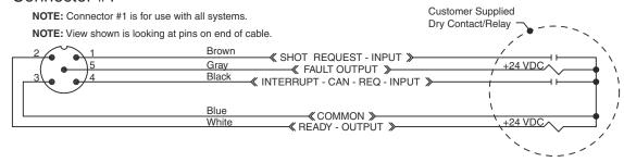
Fig. 32: External Control Interface Electrical Diagram
